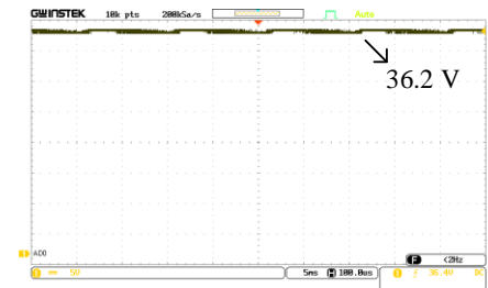
Fig. 12. The output voltage when the primary current is 200 A
