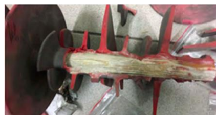
Fig. 1. Broken composite insulator caused by internal conductive defects
