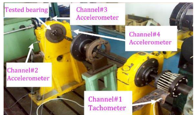
Fig. 2. The test rig of the aero-engine rotor-bearing fault simulator
