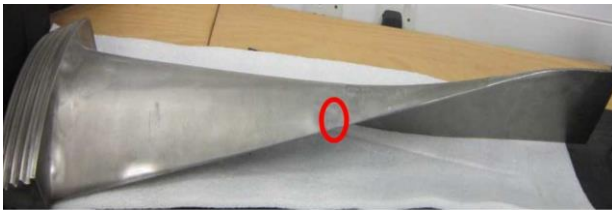
Fig. 6. Thermal fatigue crack of a steam turbine blade
